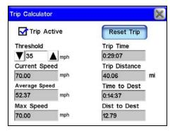
Pressing the Reset Trip button will reset all on-screen values to zero.
